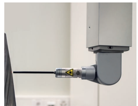
HP-O Flex sensor - highly accurate, fast and flexible non-contact measurements on CMMs. See page 31.
