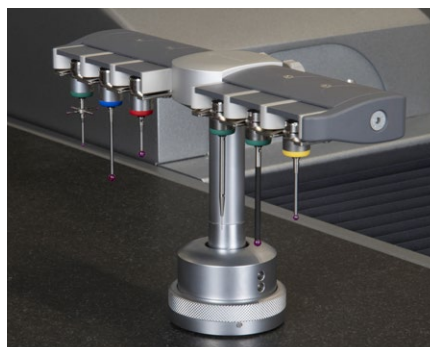
HR-MP probe module changer rack - exchange of HP-TM or HP-THD modules during part programs. See page 34.
