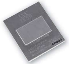
Standard Ra = 2,97 \mu\text{m}
