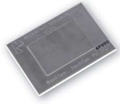
Standard Ra = 0,50 \mu\text{m}
