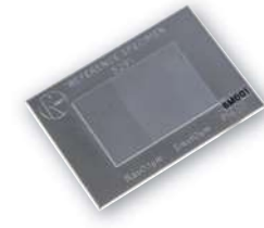
Standard Ra = 0,10 \mu\text{m}
